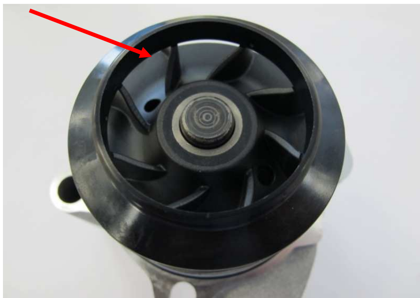
Pic.5: 24-1090/PA1090: 8 blades impeller with high performance geometry (blades double curved) that is able to provide higher flow rate respect 24-0905/PA905.
